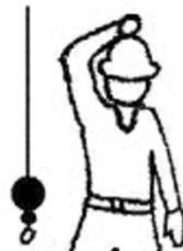
**USE MAIN HOIST** – A hand taps on top of the head. Then regular signal is given to indicate desired action.
