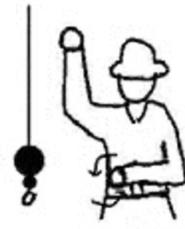
**CRAWLER CRANE TRAVEL, ONE TRACK** – Indicate track to be locked by raising fist on that side. Rotate other fist in front of body in direction that other track is to travel.
