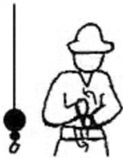
**CRAWLER CRANE TRAVEL, BOTH TRACKS** – Rotate fists around each other in front of body; direction of rotation away from body indicates travel forward; rotation towards body indicates travel backward.
