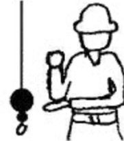
**USE AUXILIARY HOIST (whipline)** – With arm bent at elbow and forearm vertical, elbow is tapped with other hand. Then regular signal is used to indicate desired action.
